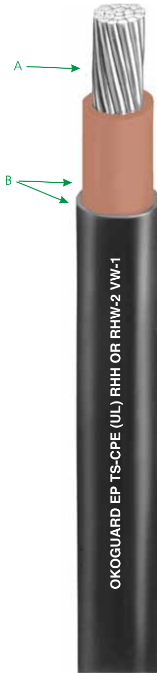
A Uncoated Copper Conductor B Composite Okoguard—Okolon TS-CPE Insulation
